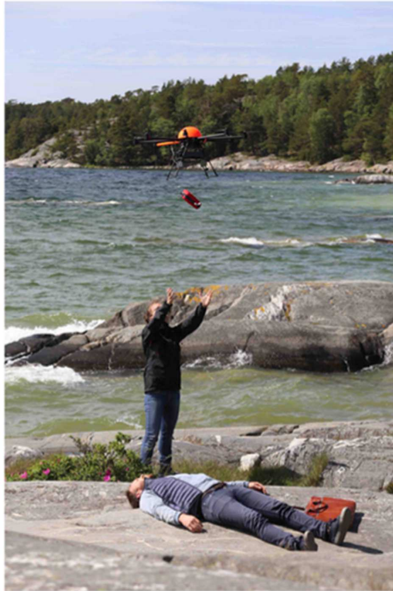
Fig. 4 AED delivery using an UAV system. Delivery of an AED in simulated OHCA from 3 m altitude using latch-release from an UAV
